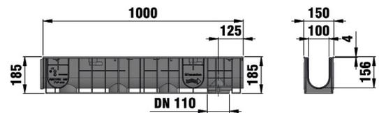
SERVICE CHANNEL RECYFIX STANDARD 200 in polipropilene Classe A 15
